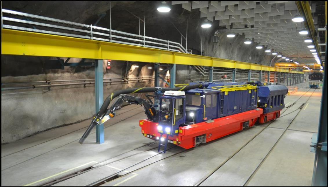
**Minevac 8000** is a vacuum-based suction machine for cleaning jobs in mines or in industrial areas where there are heavily contaminated track.
